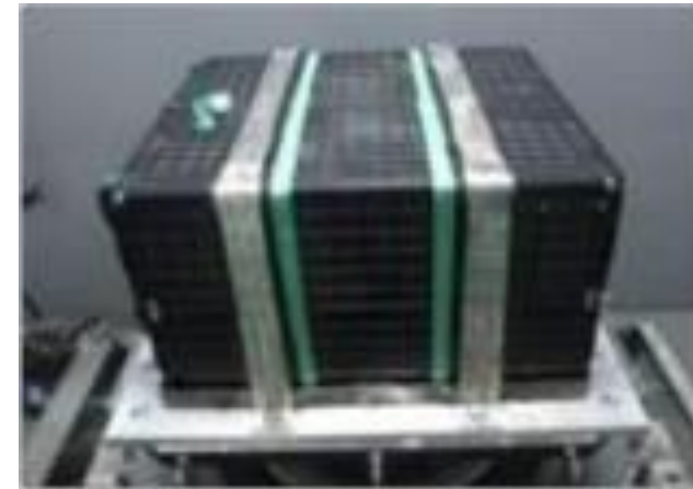
Vibration Testing 10-2000 Hz range, 8hrs
