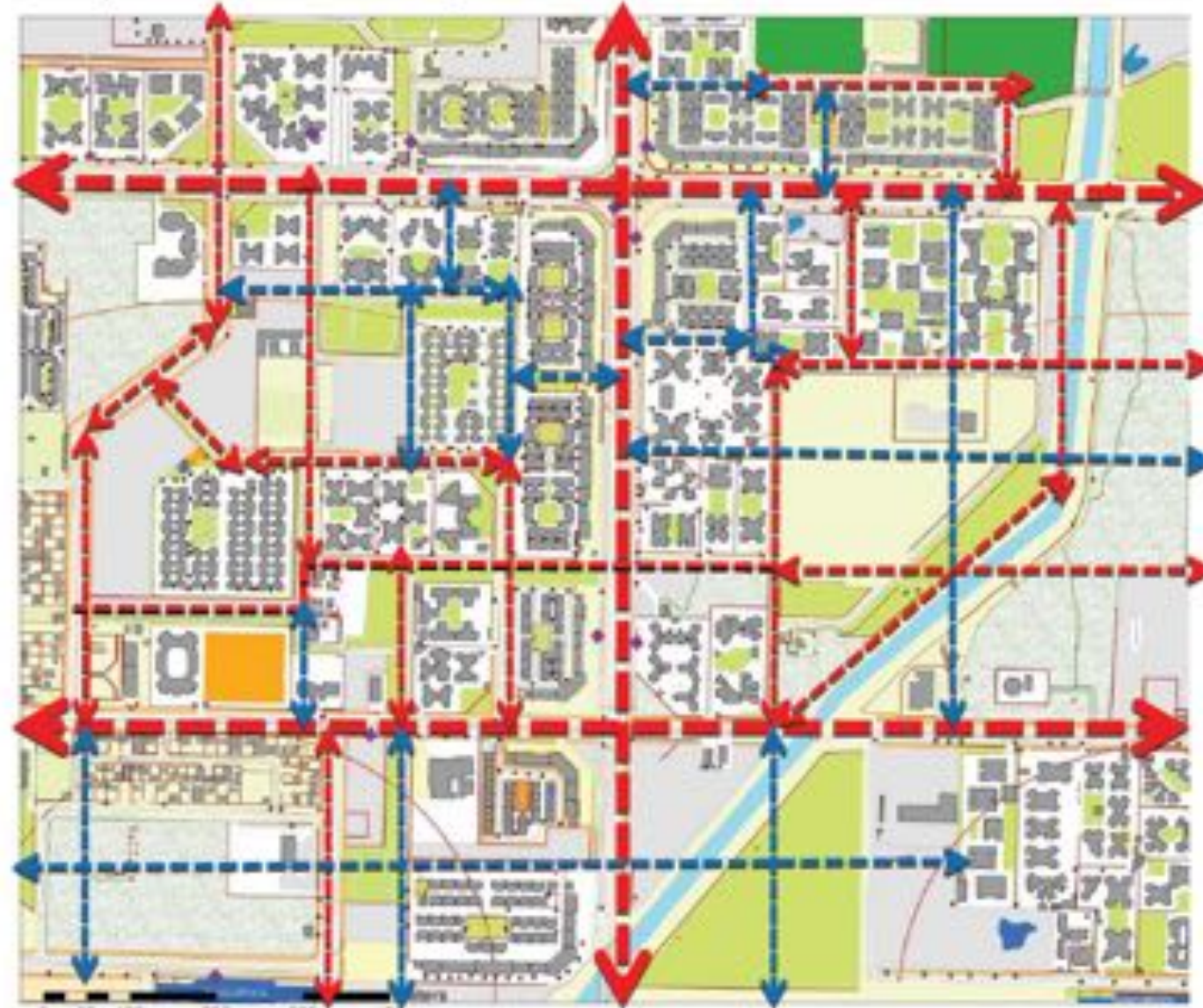
Example: Dwarka - Proposed Retrofitted Street Grid
